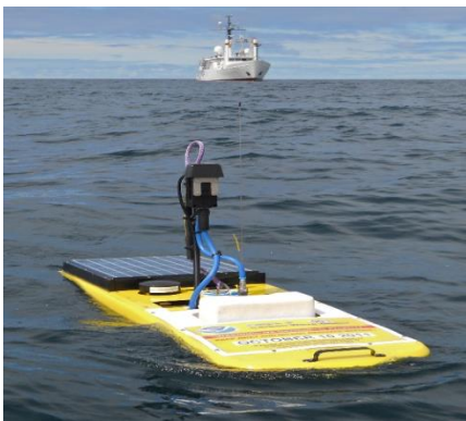
Fig. 6. The wave-driven surface robot applied in sea area surveillance
