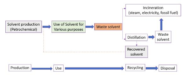
Fig. 1. System model of the solvent assessment using the life-cycle assessment method [12]
