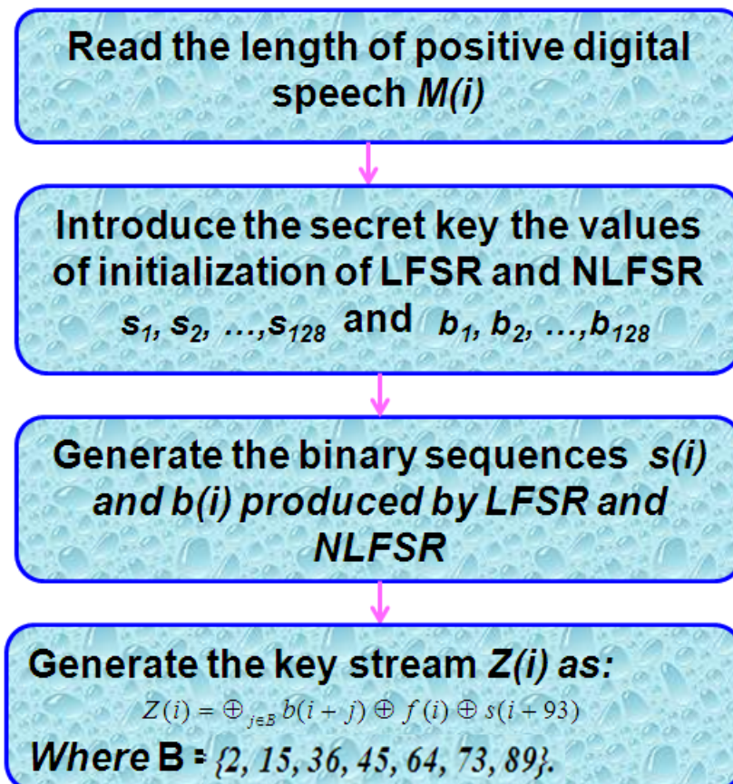
Figure 6: KSG Flow Chart of Modified Grain-128.
