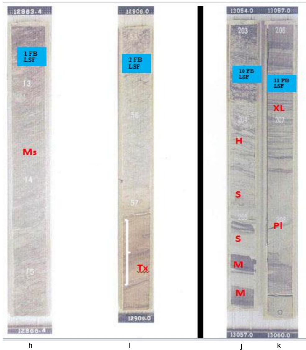
Fig. 9h-k. Interbedded sandstone/mudstone facies. Fine- very fine grained silty, laminated and bioturbated heterolithic sandstone. Bioturbated sandy mudstone facies with bioturbation intensity reducing from h-k. Note the contact between the overlying highly bioturbated heterolithic interval and the laminated tidal channel facies towards 12909.0ft (Fig. 9i). M: Mudstone, S: sandstone bed, Ms: Silty Mudstone, H: hummocky cross stratification, PI: Planolite, XL: Cross laminations with mud drapes
