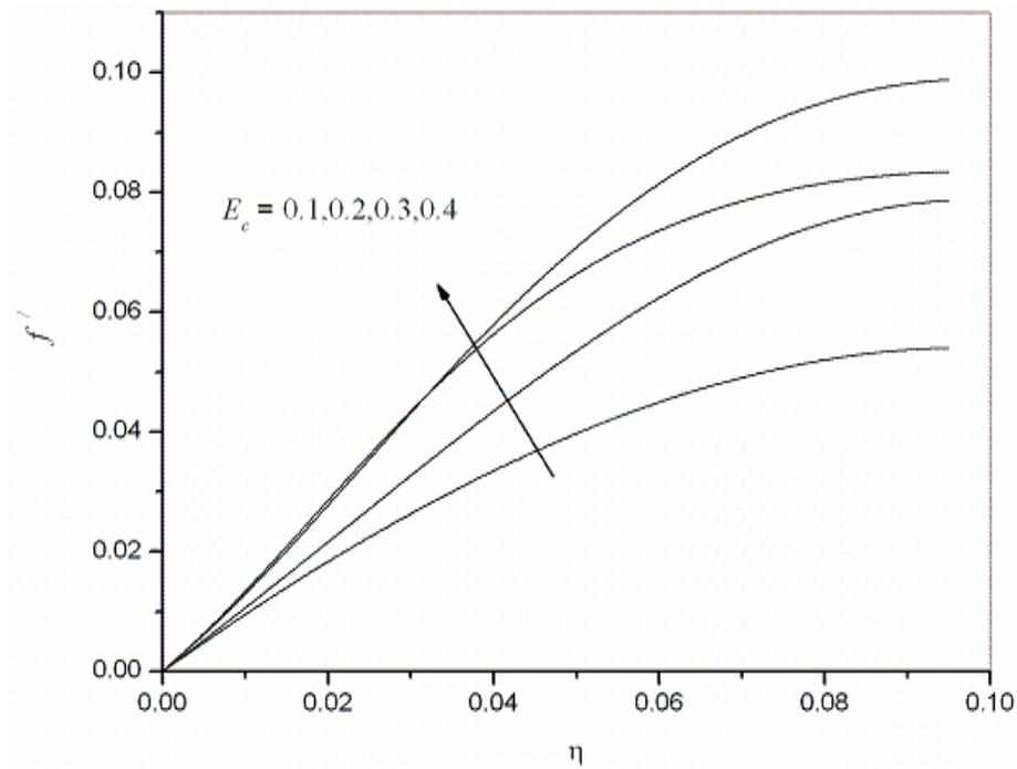
Fig. 4. Velocity profiles for different Eckert parameters  $E_c$  with  $S_r = 0.001, D_f = 10.0$
