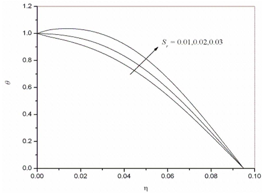
Fig. 6. Temperature profiles for different Soret parameters with  $D_f = 10.0, N = 1$ .
