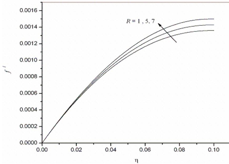
Fig. 5. Velocity profiles for different values of  $R$  with  $S_r = 0.001, D_f = 10.0, N = 1, E_c = 0.5, Le = 2$
