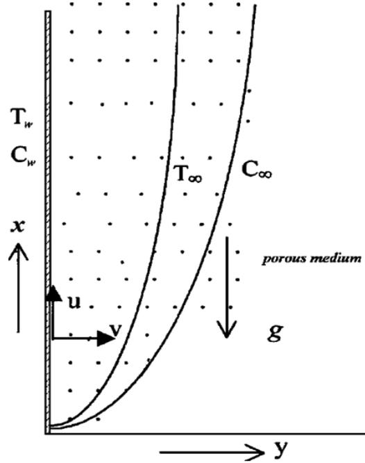
Fig. 1. Flow model and physical coordinate system
