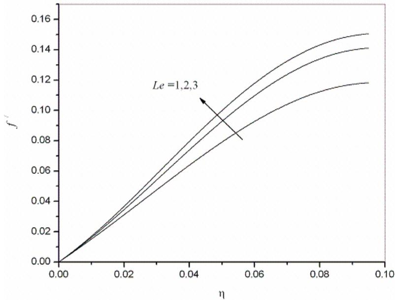
Fig. 3. Velocity profiles for different  $Le$  with  $S_r = 0.001, D_f = 10.0, N = 1$
