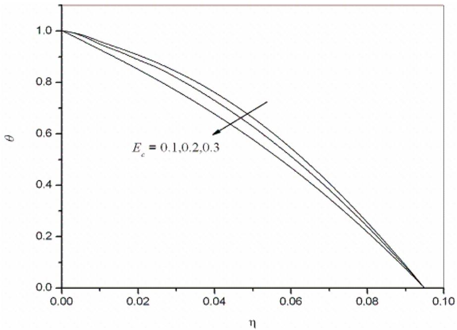
Fig. 7. Temperature profiles for different Eckert parameters  $E_c$  with  $S_r = 0.001, D_f = 10.0$
