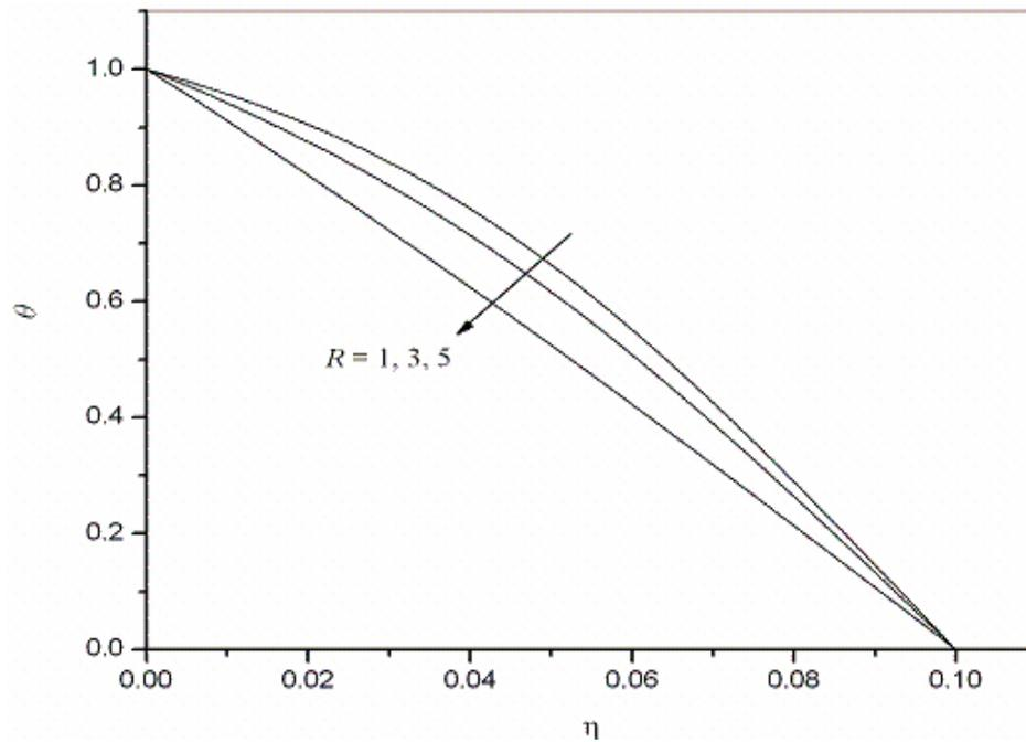
Fig. 8. Temperature profiles for different values of  $R$  with  $S_r = 0.001, D_f = 10.0, N = 1, E_c = 0.5, Le = 2$
