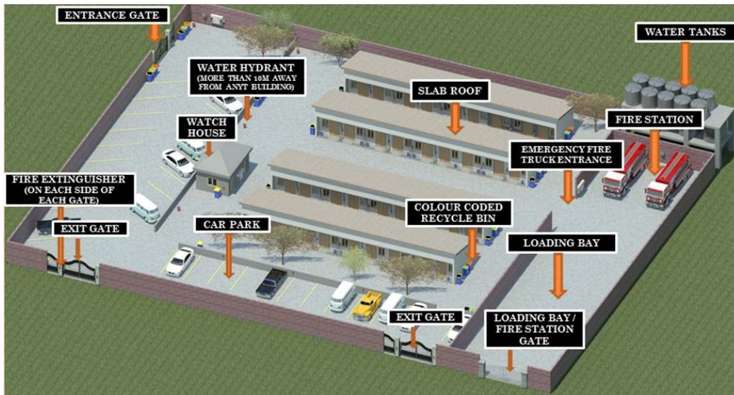
Fig. 2B. 3D dimensional view showing typical plan of an ideal market that will curb market fire
