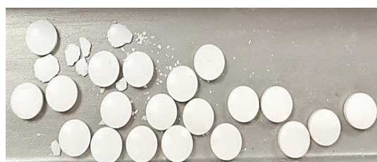
Fig. 1. Tablet capping observed in formulation 1
