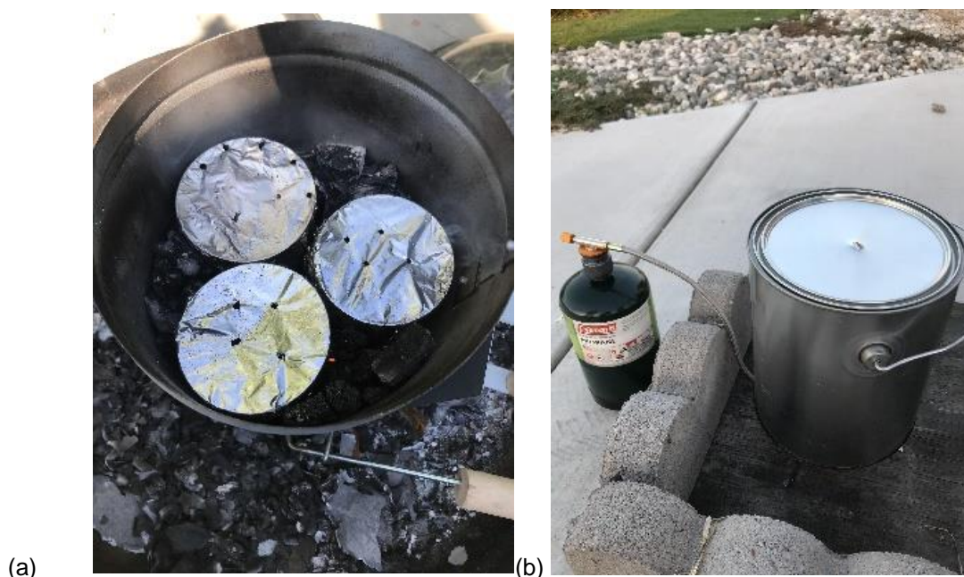
Fig. 1. Photographs showing the carbonization setup: (a) chimney starter configuration, (b) gas burner configuration
