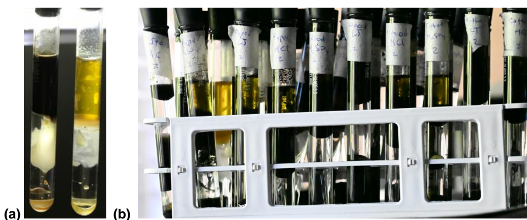
Fig. 9. (a) Control samples of 5 mL of used motor oil and olive oil and (b) AC samples in olive oil after testing for 2 weeks. Case A 10 can be seen on the far left for the commercially available activated carbon (CAC)
