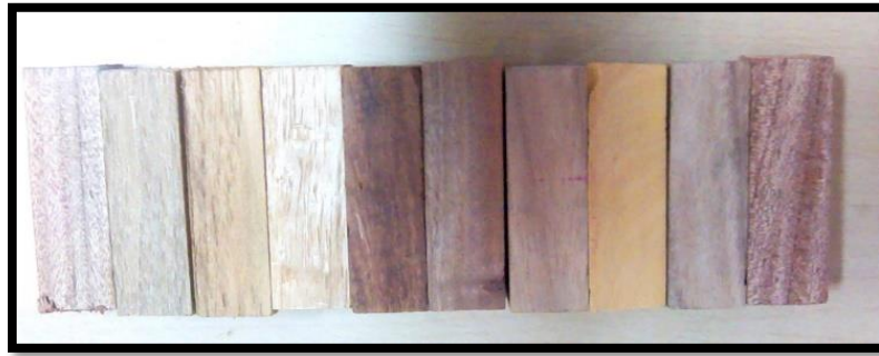
Fig. 3. Prepared specimens for hardness test
