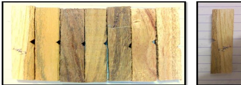
Fig. 5. Prepared specimens for impact test
