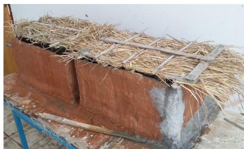
Fig. 5. Finally covering the structure with straw materials
