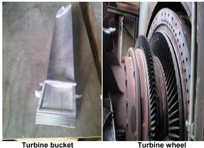
Fig. 18. The arrangement of the turbine bucket arranged radially, forms the turbine wheel
