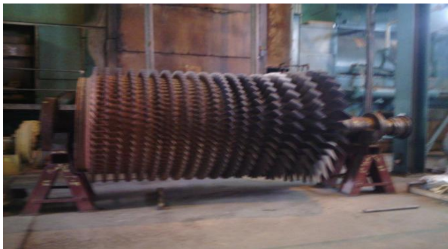
Fig. 5. Compressor rotor and blades
