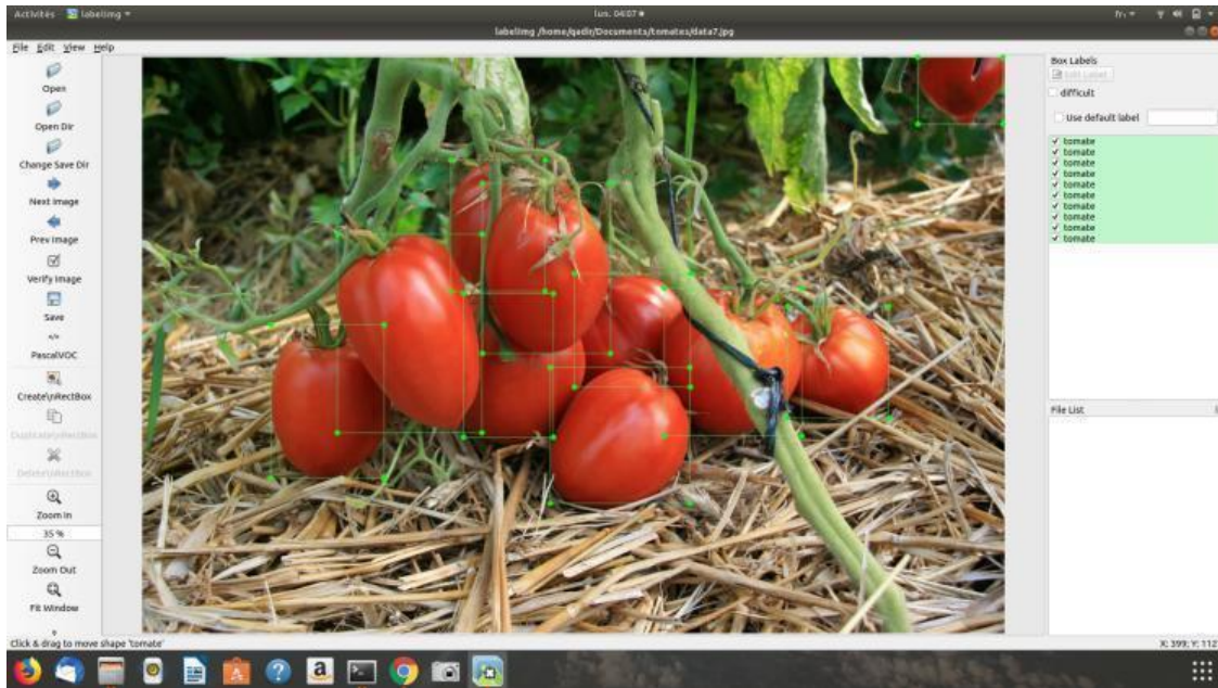
Fig. 10. Labeling of tomatoes with the labelimage tool
